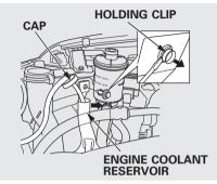
(Passenger's side) Use a flat-tip screwdriver to remove the holding clip from the engine coolant reserve tank, and then remove the engine coolant reserve tank.
