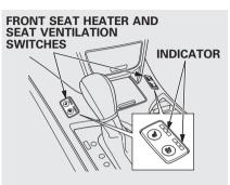
The ignition switch must be in the ON (II) position to use the heaters and the air ventilation system.
