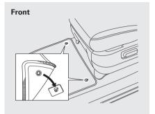
The floor mats that came with your vehicle hook over the floor mat anchors. This keeps the floor mats from sliding forward, possibly interfering with the pedals, or backwards, making the front passenger's weight sensors ineffective.
