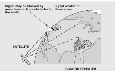
The XM satellites are in orbit over the equator; therefore, objects south of the vehicle may cause satellite reception interruptions. To help compensate for this, ground-based repeaters are placed in major metropolitan areas.
