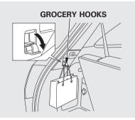
Your vehicle also has a grocery hook on each side panel in the cargo area. They are designed to hold light items. Heavy objects may damage the hook. Make sure any items put on each hook weigh less than 6.5 lbs (3 kg).
