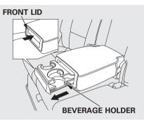
To open the beverage holder, press and release the front lid. To close, press the lid again until it latches. When you put back the armrest in the center seat-back, make sure the lid is closed properly.
