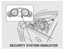
Once the security system is set, opening any door, the tailgate, or the hood without using the key or the remote transmitter, will cause the alarm to activate. It will also activate if the audio unit is removed from the dashboard or the wiring is cut. The security system will not set if the hood, tailgate, or any door is not fully closed. If the system will not set, check that the doors, the tailgate and the hood are fully closed.
