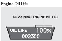
To see the remaining engine oil life displayed on the multi-information display as a percentage, turn the ignition switch to the ON (II) position. Make sure the display shows blank, SH-AWD and tire pressure, and then press the SEL/RESET button on the steering wheel repeatedly until the engine oil life appears (see page 77).
