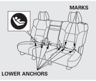
When you install a child seat in the second row seating position, use the lower anchors as shown in the illustration. You can install up to three child seats at a time with LATCH.
