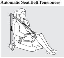
For added protection, the front seat belts are equipped with automatic seat belt tensioners. When activated, the tensioners immediately tighten the belts to help hold the driver and a front passenger in position. The tensioners can be activated during a collision in which the front airbags *do not deploy.* In this case, the airbags would not be needed, but the extra tension in the seat belt could be helpful.
