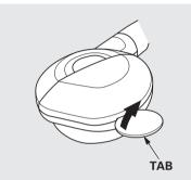
Each headphone uses one AAA battery. The battery is under the cover on the left earpiece. To remove the cover, insert a coin in the slot and twist it slightly to pry the cover away from the earpiece. Pull the cover outward, and pivot it out of the way.
