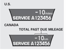
When you press the SEL/RESET button to select the engine oil life, the message "SERVICE", along with the maintenance item code and the total negative mileage after the oil life became 0%, will be displayed on the lower part of the multi-information display.
