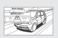
Rotate the interface dial to select each number, then press the ENTER button. Press the  $\blacktriangleright$  button when you have finished inputting the number. If you want to delete a number, press the  $\triangleleft$  button, and if you want to change the input order of a number, press the  $\blacktriangle$  button.
