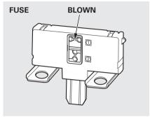
3. Check each of the large fuses in the under-hood fuse boxes by looking through the top at the wire inside. Removing these fuses requires a Phillips-head screwdriver.
