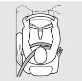
If you ever have a moderate to severe side impact, sensors will detect rapid acceleration and signal the control unit to instantly inflate either the driver's or the passenger's side airbag and activate the seat belt tensioner on the affected side. Only one airbag will deploy during a side impact. If the impact is on the passenger's side, the passenger's side airbag will deploy even if there is no passenger.
