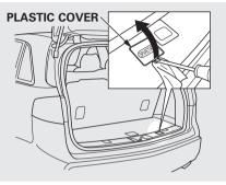
7. The spare tire is stored underneath the rear cargo area. Remove the plastic cover on the cargo area lining to access the shaft for the spare tire hoist.
