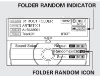
This feature, when activated, plays all files in the current folder in random order. To activate folder random play, push the interface selector down while playing a disc. Turn the interface dial to select Random on the AUDIO MENU, and press ENTER on the interface selector. Turn the interface dial to select the folder random icon, and press ENTER on the interface selector. To turn this feature off, turn the interface dial to select the OFF icon, and press ENTER on the interface selector.
