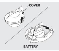
Remove the battery. Install the new battery in the earpiece as shown in the diagram next to the battery slot. Slide the cover back into place on the earpiece, then press down on the back edge to lock it in place. **Auxiliary Input Jacks**
