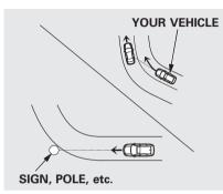
Because of the road condition (curved, winding, etc.) or the state of your vehicle (turning angle, lane position, etc.), CMBS can sometimes mistake a stationary object (light pole, traffic sign, guard rail, etc.) as a vehicle ahead of you and temporarily operate. This is normal.
