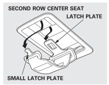
Pull out the small latch plate and the latch plate from each holding slot in the ceiling, and pull out the seat belt to extend it.
