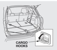
The four hooks on the side panels can be used to install a net for securing items. Each hook is designed to hold up to 50 lbs (23 kg) of weight.
