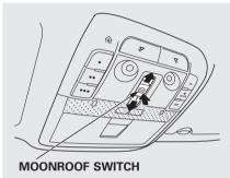
To open the moonroof fully, pull back the moonroof switch firmly. The moonroof opens all the way. To stop the moonroof from opening fully, push the switch briefly.
