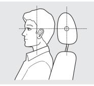
They are most effective when you adjust them so the center of the back of the occupant's head rests against the center of the restraint.
