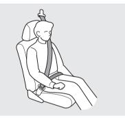
Position the lap part of the belt as low as possible across your hips, then pull up on the shoulder part of the belt so the lap part fits snugly. This lets your strong pelvic bones take the force of a crash and reduces the chance of internal injuries. If necessary, pull up on the belt again to remove any slack, then check that the belt rests across the center of your chest and over your shoulder.
