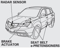
The CMBS consists of a radar sensor in the front grille, a brake actuator in the engine compartment, an indicator on the instrument panel, seat belt e-pretensioners on the front seats, and an on/off button on the dashboard.
