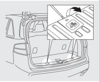
Each third row seat has a tether anchorage point on the tailgate sill.
