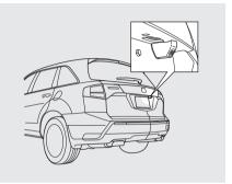
For the best picture, always keep the rearview camera clean, and do not cover the camera lens. To avoid scratching the lens when you clean it, use a moist, soft cloth.
