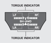
The SH-AWD torque distribution monitor on the multi-information display shows you the amount of torque being sent to the wheels. Each wheel-right front (RF), left front (LF), right rear (RR), and left rear (LR)-has its own torque indicator. Each torque indicator is displayed as a bar graph divided into 5 segments. The number of segments represents the amount of torque distributed to each wheel.
