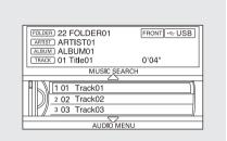
You can also select a folder or file from the list by using the interface dial. Press the AUDIO button to show the audio display on the navigation screen. Use the interface dial to highlight the file, then press ENTER to set your selection.
