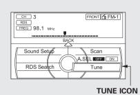
**TUNE** – Use the TUNE knob to tune the radio to a desired frequency. Turn the knob right to tune to a higher frequency, or left to tune to a lower frequency. To tune with the interface dial, push the selector down, and turn the knob to TUNE. Then press ENTER on the selector, and turn the knob to the desired frequency. To exit the TUNE mode, press ENTER on the interface selector, then push the interface selector up to go back.
