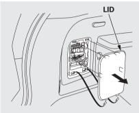
If the fuel fill door release button does not work, use the release lever inside the rear fuse box lid in the cargo area.
