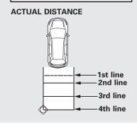
The camera display has parking guide lines that indicate distance from your vehicle.
