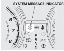
If there is a problem with your vehicle, for example, the engine oil level is low or a door is not fully closed, the multi-information display will show you the problem. It does this by interrupting the current display with one or more messages. The system message(s) triggers the appropriate indicator(s) on the instrument panel, including the system message indicator, to come on. The system message indicator does not go off until the problem(s) is corrected.
