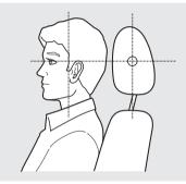
Adjust the driver's head restraint so the center of the back of your head rests against the center of the restraint.
