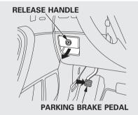
To apply the parking brake, push the pedal down with your foot. To release it, pull the release handle fully. The parking brake indicator on the instrument panel should go out when the parking brake is fully released (see page 67).
