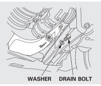
2. Open the hood, and remove the engine oil fill cap. Remove the oil drain bolt and washer from the bottom of the engine. Drain the oil into an appropriate container.
