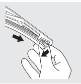
2. Slide the blade out of the wiper arm.
