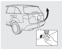
To open the tailgate, push up inside the handle, then lift up. To close the tailgate, use the inner handle to pull it down, then press down on the back edge.
