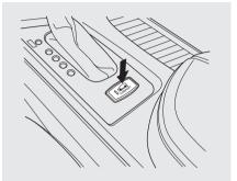
To switch between comfort and sport mode, press and release the active damper system button located on the center console to choose the desired mode.
