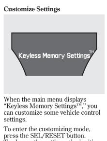
press the SEL/RESET button. To change the settings, the ignition switch must be in the ON (II) position, and the vehicle must be stopped with the transmission in Park. If you turn the ignition switch to the ACCESSORY (I) or the LOCK (0) position, or move the shift lever out of Park, the display will change to the normal screen.
