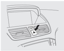
Push the button between the center vents to turn on the hazard warning lights (four-way flashers). This causes all four outside turn signals and both indicators in the instrument panel to flash. Use the hazard warning lights if you need to park in a dangerous area near heavy traffic, or if your vehicle is disabled. **Rear Window Defogger**
