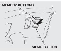
3. Press and release the MEMO button on the control panel. You will hear a beep. Immediately press and hold one of the memory buttons (1 or 2) until you hear two beeps. The indicator in the memory button will come on. The current positions of the driver's seat, steering wheel, and outside mirrors are now stored. Doing any of the following after pressing the MEMO button will cancel the storing procedure.
