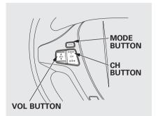
Three controls for the audio system are mounted in the steering wheel hub. These let you control basic functions without removing your hand from the wheel.
