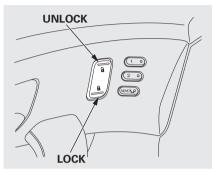
To lock all doors and the tailgate, press the bottom of the master door lock switch on either front door, pull the lock tab above the driver's door handle, or use the key on the outside lock on the driver's door.
