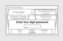
When you select and enter "Yes," the display changes as shown above. To change the level, you need to enter your four digit password. Select the number for the first digit by turning the interface dial, and enter it by pressing the ENTER button. Repeat this until all four digits are filled. Press the ▶ button on the control panel.
