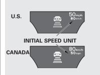
If you change the speed unit measurement from the factory default setting, the initial speed unit measurement is shown under the current unit.
