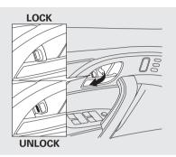
The lock tab on any passenger's door locks and unlocks that door.
