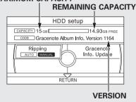
You can check the HDD Audio capacity and remaining space as well as the Gracenote Music Recognition Service (CDDB) version included with the navigation system on the HDD Setup screen.
