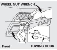
3. Screw the towing hook into the hole, and tighten it with the wheel nut wrench.
