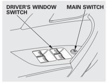
Turn the ignition switch to the ON (II) position to raise or lower any window. To open a window, push the switch down and hold it. Release the switch when you want the window to stop. Pull back on the switch and hold it to close the window. The windows will operate for up to 10 minutes after you turn off the ignition switch. Opening either front door cancels this function.
