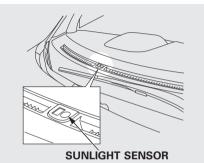
To regulate the interior temperature and humidity, the climate control system has two sensors. A sunlight sensor is located in the top of the dashboard and a temperature/ humidity sensor is next to the steering column. Do not cover the sensors or spill any liquid on them.
