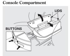
Your vehicle is equipped with a front seat armrest pad that is also a console compartment. To open the console compartment fully, push both buttons at the front of the compartment.
