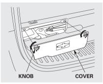
5. The tools and jack are under the cargo area behind a cover on the driver's side. Remove the cover by turning the knobs counterclockwise, then pulling out the cover.
