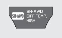
If the SH-AWD indicator blinks while driving, it indicates the differential temperature is too high. You will also see an "SH-AWD DIFF TEMP. HIGH" message on the multiinformation display. If this happens, pull to the side of the road when it is safe, shift to Park, and let the engine idle until the indicator goes out. If the indicator does not go out, take your vehicle to a dealer to have it checked. SH-AWD SYSTEM
