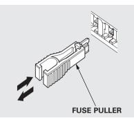
4. Check the smaller fuses in the under-hood fuse boxes and rear fuse box, and all the fuses in the interior and rear fuse boxes by pulling out each one with the fuse puller provided in the primary under-hood fuse box.
