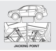
12. Place the jack under the jacking point nearest the tire you need to change. Turn the end bracket clockwise until the top of the jack contacts the jacking point. Make sure the jacking point tab is resting in the jack notch.
