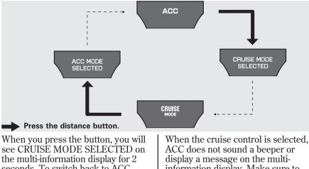
the multi-information display for 2 seconds. To switch back to ACC. press and hold the distance button again for 1 second.
