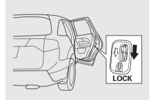
The childproof door locks are designed to prevent children seated in the rear from accidentally opening the rear doors. Each rear door has a lock lever near the edge. With the lever in the LOCK position (lever is down), the door cannot be opened from the inside regardless of the position of the lock tab. To open the door, push the lock tab forward and use the outside door handle.
