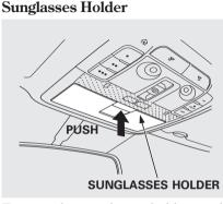
To open the sunglasses holder, push on the lid. It will unlatch and swing down. To close it, push it until it latches. Make sure the holder is closed while you are driving.
