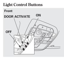
Your vehicle has the light control buttons on the front ceiling. With these buttons, you can select three positions: OFF, Door (door activated position), and ON. To select a position, press the appropriate button.
