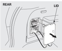
The rear fuse box is located at the left side of the cargo area.
