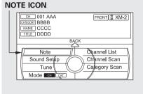
To replay and see the stored file, press the AUDIO button to select the audio display on the navigation screen.
