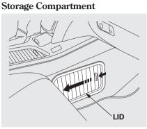
The storage compartment with a sliding lid is at the left-side foot of the front passenger seat.
