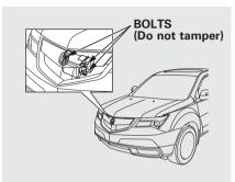
Always keep the radar sensor cover clean. If it gets dirty, clean it with water or a mild detergent. Never use chemical solvents or polishing powder
