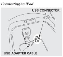
1. Unclip the USB connector by pulling it up, and pull out the USB adapter cable in the console compartment.
