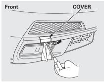
1. To remove the cover, put cloth on the edge of the cover and carefully pry with a small flat-tip screwdriver or a metal fingernail file.
