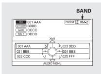
**Preset** – You can store up to 12 preset channels using the six preset buttons. Each button stores one channel from the XM1 band and one channel from the XM2 band.
