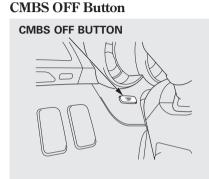
To switch the CMBS off, press the CMBS OFF button on the dashboard for about 1 second. When you do this, a beeper sounds, a CMBS indicator on the instrument panel comes on, and a CMBS OFF message appears on the multiinformation display. To switch the system back on, press the button again for about 1 second. When you turn the ignition switch to the ON (II) position, the CMBS will be in the previously selected on or off setting.
