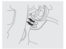
Adjust the brightness of the instrument panel by pressing the + or - button. Press the + button to increase the brightness and the - button to decrease it. The brightness can be set differently for when the headlights are on, and when they are off.
