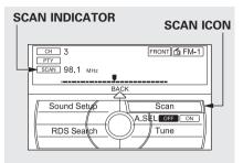
**SCAN** – The SCAN function samples all stations with strong signals on the selected band. To activate it, press the SCAN button, then release it. To scan with the interface dial, push the selector down, and turn the interface dial to select Scan, then press ENTER on the interface selector.
