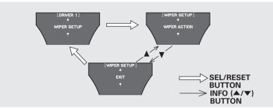
Here is one custom setting for the wiper setup:
