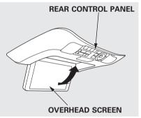
Press the REAR PWR button in the front panel or press the  $\bigcirc$  button in the rear control panel when REAR PWR is on. The overhead screen will open to the position it was last set. You can tilt the screen at nine different angles from 90 to 130 degrees using the tilt button in the rear control panel. The default setting is 100 degrees.
