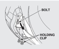
2. Remove the bolt and use the flattip screwdriver to remove the holding clips located under the front bumper.
