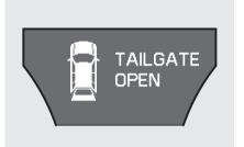
When the tailgate is not tightly closed, the "TAILGATE OPEN" message will come on.
