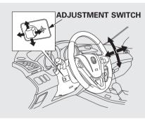
Move the steering wheel in, out, up, or down by pushing and holding the adjustment switch in that direction. Release the switch when the steering wheel reaches the desired position. Make sure the steering wheel points towards your chest, not toward your face, and that you can see the instrument panel gauges and indicators.
