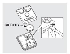
3. Place a cloth on the edge of the keypad, and remove the upper half by carefully prying on the edge with a small flat-tip screwdriver.
