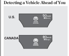
When the system detects a vehicle ahead of you, a beeper sounds once and a solid-line vehicle icon appears on the multi-information display.
