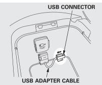
1. Unclip the USB connector by pulling it up, and pull out the USB adapter cable in the console compartment.
