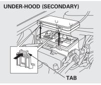
The secondary fuse box is on the passenger's side.
