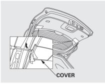
1. Open the tailgate. Place a cloth on the edge of the light assembly cover. Remove the cover by carefully prying in the notch on its middle edge with a flat-tip screwdriver.
