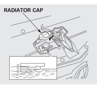
3. Remove the radiator cap by pushing down and turning counterclockwise.
