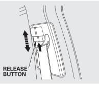
The front seats have adjustable seat belt anchors. To adjust the height of an anchor, squeeze the release button and slide the anchor up or down as needed (it has four positions). *Never place the shoulder portion of a lap/shoulder belt under your arm or behind your back.* This could cause very serious injuries in a crash.
