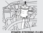
(Passenger's side) Remove the power steering reserve tank from the stay brackets.
