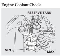
Look at the coolant level in the radiator reserve tank. Make sure it is between the MAX and MIN lines. If it is below the MIN line, see **Adding Engine Coolant** on page 514 for information on adding the proper coolant.
