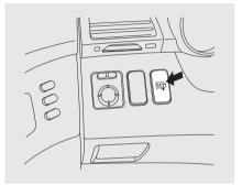
The headlight washers can be operated at any time by pressing the headlight washer button located next to the steering wheel column. The headlights must be turned on to use this button. In addition, the headlight washer operates without pressing the button the first time you turn on the windshield washers with the ignition switch in the ON (II) position. The headlight washers use the same fluid reservoir as the windshield washers.
