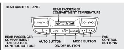
You can use the rear control panel when the indicator in the REAR button on the front control panel is on. Pressing any control button on the rear control panel turns on the rear button indicator on the front control panel.
