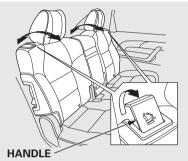
To change the seat-back angle of the seats in the second row, pull up on the handle on the outside of the seatback, and push the seat-back.
