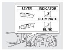
The BSI alert indicator starts to blink as a reminder if you move the turn signal lever in the direction of the detected vehicle.
