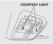
The courtesy lights between the front map lights come on when the parking lights are turned on. To adjust its brightness, press either of the instrument panel brightness control buttons (+ or -) with the ignition switch in the ON (II) position.
