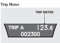
This meter shows the number of miles (U.S.) or kilometers (Canada) driven since you last reset it. There are two trip meters: Trip A and Trip B. Each trip meter works independently, so you can keep track of two different distances.
