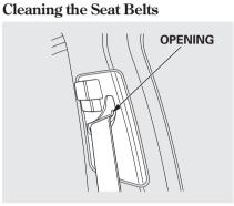
If your seat belts get dirty, use a soft brush with a mixture of mild soap and warm water to clean them. Do not use bleach, dye, or cleaning solvents. Let the belts air-dry before you use the vehicle. Dirt build-up around the openings of the seat belt anchors can cause the belts to retract slowly. Wipe the openings with a clean cloth dampened in mild soap and warm water or isopropyl alcohol.
