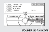
This function samples the first file in each folder within the USB flash memory device.
