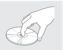
Handle a disc by its edges; never touch either surface. Do not place stabilizer rings or labels on the disc. These, along with contamination from finger prints, liquids, and felt-tip pens, can cause the disc to not play properly, or possibly jam in the drive.
