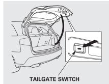
The tailgate can also be closed by pressing the button on the tailgate. If you press the button again while the tailgate is closing, you will hear three beeps, and the tailgate will stop moving, reverse direction, and stop at the fully opened position.
