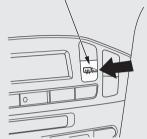
The outside mirrors are heated to remove fog and frost. With the ignition switch in the ON (II) position, turn on the heaters by pressing the button. The indicator in the button comes on as a reminder. Press the button again to turn the heaters off. Pressing this button also turns the rear window defogger on and off.
