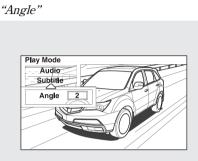
To change the view angle, highlight "Angle" from the play mode menu with the  $\nabla$  or  $\blacktriangle$  button. You can see the available angle options with the interface dial.
