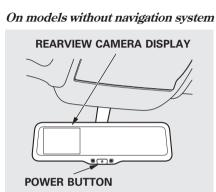
You can turn the camera display on and off by pressing the power button when the shift lever is in reverse. The camera display turns on everytime you shift to reverse, even if you turned it off the last time.
