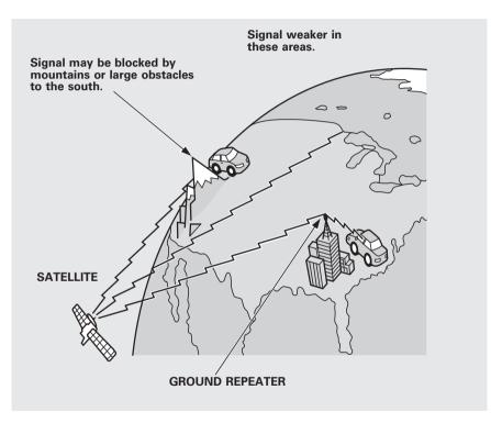
The XM satellites are in orbit over the equator; therefore, objects south of the vehicle may cause satellite reception interruptions. To help compensate for this, ground-based repeaters are placed in major metropolitan areas. Satellite signals are more likely to be blocked by tall buildings and mountains the farther north you travel from the equator.
