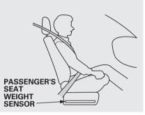
The passenger's advanced front airbag system has weight sensors under the seat. Although Acura does not encourage carrying an infant or small child in front, if the sensors detect the weight of an infant or small child (up to about 65 lbs or 29 kg), the system will automatically turn the passenger's front airbag off. Be aware that objects placed on the passenger's seat can also cause the airbag to be turned off.
