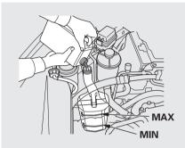
If the coolant level in the reserve tank is at or below the MIN line, add coolant to bring it up to the MAX line. Inspect the cooling system for leaks. Always use Honda Long-life Antifreeze/Coolant Type 2. This coolant is pre-mixed with 50 percent antifreeze and 50 percent water. Never add straight antifreeze or plain water.
