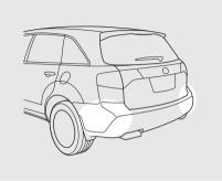
Radar sensors, located underneath each corner of the rear bumper, detect objects. Do not cover this area with labels or stickers of any kind. Always keep this area is free of any kind of dirt every time you get in the vehicle.
