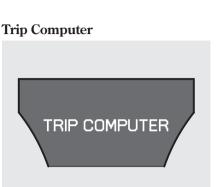
When the main menu displays "TRIP COMPUTER", pressing the SEL/ RESET button changes the display to "AVERAGE FUEL A/RANGE" to "AVERAGE FUEL B/RANGE" and to "AVERAGE SPEED/ELAPSED TIME".
