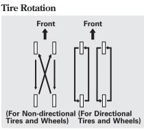
To help increase tire life and distribute wear more evenly, rotate the tires according to the maintenance messages displayed on the multi-information display. Move the tires to the positions shown in the illustration each time they are rotated. If you purchase directional tires, rotate only front-to-back.
