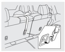
For the center seat, lower the head restraint, then route the tether strap over the head restraint and seat-back.
