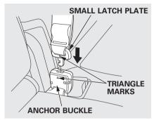
Line up the triangle marks on the small latch plate and anchor buckle when reattaching the belt and buckle.
