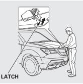
2. Put your fingers under the front edge of the hood near the center. Slide your hand to your left until you feel the hood latch handle. Push this handle up until it releases the hood. Lift up the hood.
