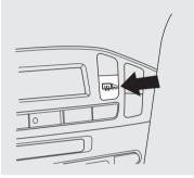
The rear window defogger will clear fog, frost, and thin ice from the window. Push the defogger button to turn it on and off. The indicator in the button lights to show the defogger is on. If you do not turn it off, the defogger will shut itself off after about 15 minutes. It also shuts off when you turn off the ignition. You have to turn it on again when you restart the vehicle. Make sure the rear window is clear and you have good visibility before starting to drive.
