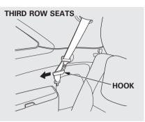
Pull out the outer shoulder belts from the hook. Both of the third-row hooks should only be used when the seat belt is detached.
