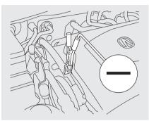
4. Connect the second jumper cable to the negative (-) terminal on the booster battery. Connect the other end to the grounding point as shown. Do not connect this jumper cable to any other part of the engine.
