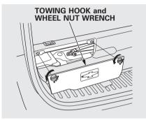
2. Remove the towing hook and wheel nut wrench located behind the cargo area cover on the driver's side.
