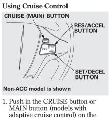
steering wheel. The CRUISE MAIN indicator or green ACC indicator (models with ACC) on the instrument panel comes on. On models with adaptive cruise control
