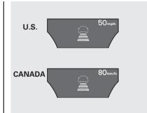
When that vehicle changes lanes or goes out of ACC range, a beeper sounds once. If there is no vehicle ahead of you within ACC range, a dotted-line vehicle icon will be on the multi-information display. To set the ACC beeper on or off, see page 96.
