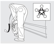
18. Tighten the wheel nuts securely in the same crisscross pattern. Have the wheel nut torque checked at the nearest automotive service facility.
