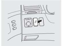
To turn the system off, press the BSI OFF button when the ignition switch is in the ON (II) position. The BSI indicator on the instrument panel glows amber, indicating that the system is turned off. The multiinformation display indicates that the system is off. To turn the system on again, press the same button. The BSI indicator on the instrument panel turns off. The multi-information display indicates that the system is on.
