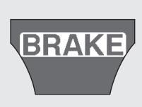
The visual alert is an amber colored BRAKE message that flashes on the multi-information display, the audible alert is a constant beeping sound. If one or more of the alerts come on, take the appropriate means to prevent a collision (apply the brakes, change lanes, etc.).
