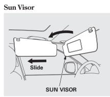
To use the sun visor, pull it down. When using the sun visor for the side window, remove the support rod from the clip, and swing it out. In this position, the sun visor can be adjusted by moving it on its slider. Do not use the extended sun visor over the inside mirror.
