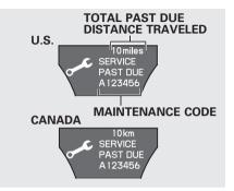
If the indicated required service is not done and the remaining engine oil life becomes 0%, the multiinformation display will show a "SERVICE PAST DUE" message, the total distance traveled after the remaining oil life became 0%, and the maintenance item code(s). This message is displayed when you drive over 10 miles (for U.S. models) or 10 km (for Canadian models) after seeing the 0% message.
