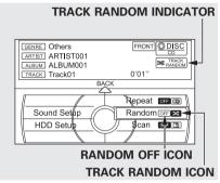
This feature plays the tracks within a disc in random order. When playing MP3, WMA or AAC format discs, all the tracks within the disc are played in random order, regardless of the configuration of the folder.
