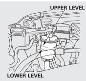
Check the level on the side of the reservoir when the engine is cold. The fluid should be between the UPPER LEVEL and LOWER LEVEL. If not add power steering fluid to the UPPER LEVEL mark.
