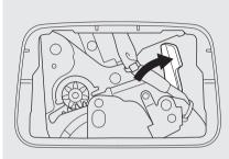
Push the release lever to the right as shown.
