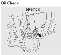
Wait a few minutes after turning the engine off before you check the oil.
