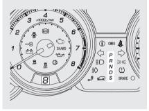
These indicators on the instrument panel show which position the shift lever is in.
