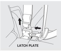
The seat belts in the second row center seat and the third row seats are equipped with detachable anchors.
