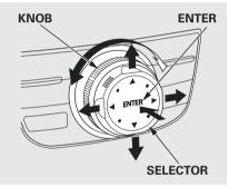
The knob turns left and right. Use it to make selections or adjustments to a list or menu on the screen. The selector can be pushed left, right, up, down, and in. Use the selector to scroll through lists, to select menus, and to highlight menu items. When you make a selection, push the center of the selector (ENTER) to go to that selection.
