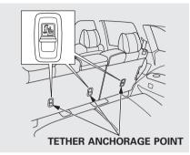
Each second row seat has a tether anchorage point behind the seat-back.
