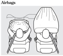
Your vehicle has a supplemental restraint system (SRS) with front airbags to help protect the heads and chests of the driver and a front seat passenger during a moderate to severe frontal collision (see page 29 for more information on how your front airbags work).
