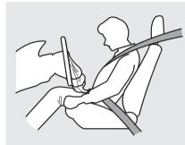
After inflating, the front airbags immediately deflate, so they won't interfere with the driver's visibility, or the ability to steer or operate other controls.
