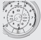
When you move the shift lever from "D" to "S" position and pull either paddle shifter, the gear position indicator displays the selected gear number.
