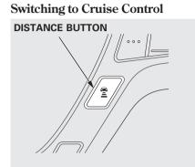
To switch from ACC to cruise control, press the distance button on the steering wheel, and hold it for 1 second.
