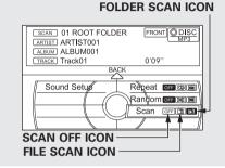
This feature samples all files in the selected folder in the order they are stored. To activate this feature, press the SCAN button. You can also select the SCAN icon with the interface dial. Push the selector down, turn the dial to select Scan on the AUDIO MENU, then press ENTER. Turn the dial to select the scan icon, then press ENTER. The system begins to play a file for about 10 seconds, and continues to sample the remaining files.
