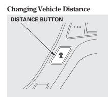
With ACC on, the distance between your vehicle and the vehicle ahead of you is controlled and maintained. You can change this distance to one of three ranges: long, middle, or short. To change the range, press the distance button. Each time you press the button, the range changes from Long, to Middle, and then to Short.
