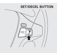
3. Press and release the SET/ DECEL button on the steering wheel, then release the accelerator pedal.
