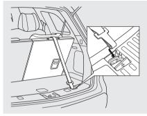
3. Remove the head restraint, then attach the tether strap hook to the anchor, making sure the strap is not twisted.
