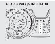
When you pull either paddle shifter, the gear position indicator shows you the selected gear number. The transmission control system monitors the accelerator pedal use and your driving conditions. When you press the accelerator pedal as in normal driving, the system judges that you are driving at a constant cruising speed without using the paddle shifters. Under these conditions, D-paddle shift mode is canceled, and the transmission automatically returns to drive mode (D).
