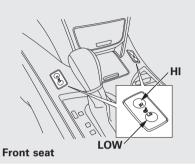
Push the front of the switch, HI, to rapidly heat up the seat. After the seat reaches a comfortable temperature, select LO by pushing the back of the switch. This will keep the seat warm.
