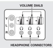
There are three headphone connectors for the third seat. passengers. Each connector has its own volume control.
