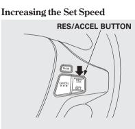
The set speed can be increased by using the RES/ACCEL button or the accelerator pedal.
