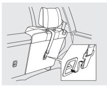
6. Attach the tether strap hook to the tether anchor, then tighten the strap as instructed by the child seat maker.
