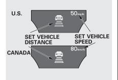
When the speed is set, it is shown along with a vehicle icon and distance bars on the multiinformation display. Refer to page 354 for how to set and change the set distance between your vehicle and the vehicle ahead of you.
