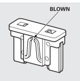
5. Look for a burned wire inside the fuse. If it is burned out, replace it with one of the spare fuses of the same rating or lower.
