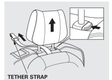
5. Lift the head restraint (see page 149), then route the tether strap through the legs of the head restraint and over the seat-back, making sure the strap is not twisted.
