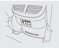
Auxiliary input jacks and headphone connectors for the rear entertainment system are on the back of the center console compartment.
