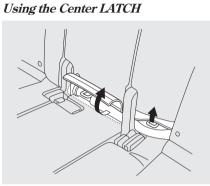
To install a LATCH-compatible child seat in the center seating position on the second row seat, use the center lower anchors as shown above.
