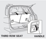
3. Unlock the seat-back by pulling the handle. Push the seat-back forward.
